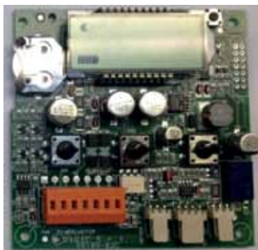
7930-24 – This board allows to drive a chlorine producer
