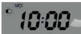
Day of the week and service icon blink to confirm Delayed Manual Regeneration
