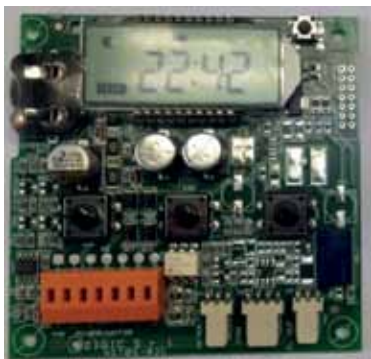
7930-23 – The standard board allows to program a dry contact relay
